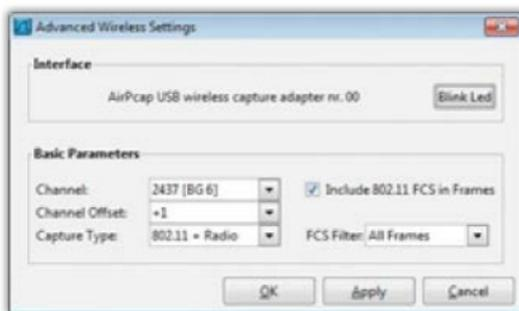
*Figure 7. Wireless Settings Dialog in Wireshark*
